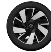
03 20" Plus machined alloy wheels (All-season tires 255/50 R20 105T) (Highline 4MOTION®)
