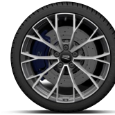
01 19" Warmenau forged alloy wheels (Summer performance tires 235/35 R19) 8J x 19 (R)
