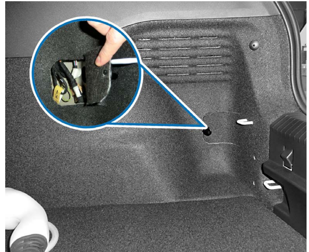
Version 1: Cut-out connection in the luggage compartment (example ID.3) behind the side panel trim until the end of 2020. The yellow flag indicates the cut-out connection.
