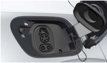
Charging socket CCS1 DC and AC (e.g. in North America, South Korea)
