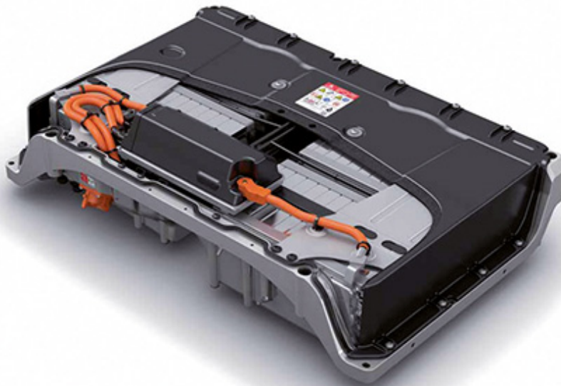
The high-voltage battery of the Passat GTE
