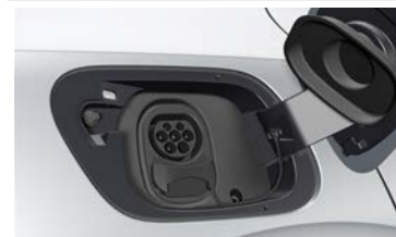
Charging socket Type 2 AC (e.g. in the EU)
