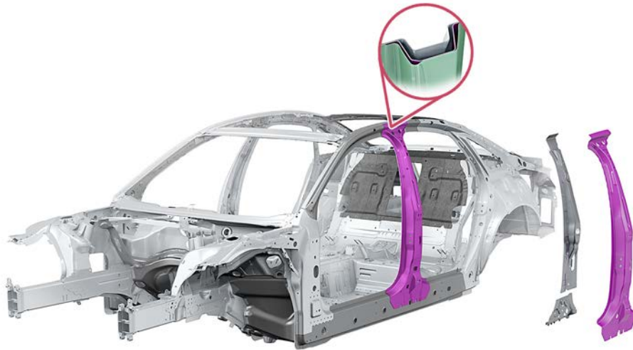
B-pillar with multi-shell structure
