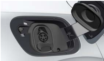
Charging socket Type 1 AC (e.g. in North America, South Korea, Japan)
