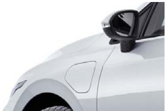
Charging flap on the Golf GTE as of 2020 (Plug-in hybrid)
