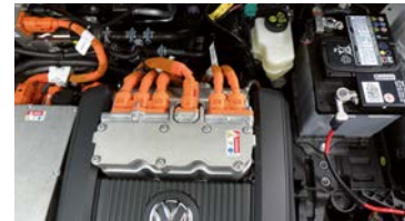
Orange high-voltage cables in the motor compartment
