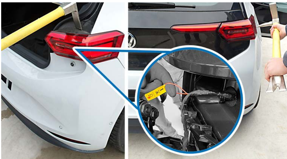
Version 2: Cut-out connection in the rear of the vehicle behind the right tail light cluster from the start of 2021 onwards.
