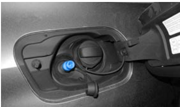
Natural gas connection at the fuel filler neck
