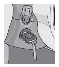
1. Turn the ignition key to the "OFF" position and remove it.
